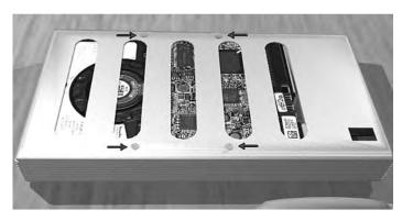
4) Hook the bottom cover in place to cover the bottom of the unit (see image below). Repeat for top cover.
